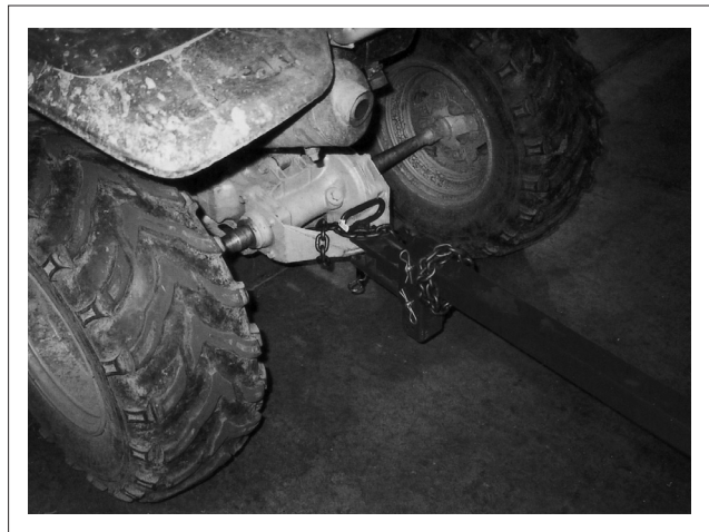
FIG. 20 LEVELLING THE FRAME
