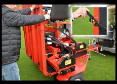
The ramp self locking mechanism provides safe transportation. Thanks to the ramp spring assisted hinge system, make it easy for the operator to lift it back up before driving to the next green.
