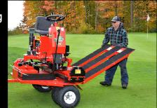
The large tire wheels prevent excessive compaction when parking next to your valuable greens. The GR-660 trailer is equiped with 4 wheels for minimum compaction.
